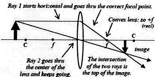
If the object is outside  $C$  ( $2f$ ) in front of a convex lens, then the image is real, reduced, and located between  $f$  and  $C$ .
