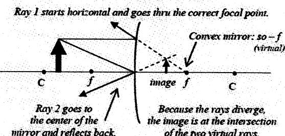
If the object is between  $f$  and  $C$  in front of a convex mirror, then the image is virtual, reduced, and located inside  $f$ .
