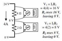
Notice V = 8 V between the resistors. Also, the total voltage used by the resistors must equal the total voltage given by the batteries: 24 volts.
