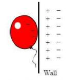
When a balloon is charged by contact (rubbed with fur) it gains electrons, becoming negative. The electrons in the wall are repelled, shifting slightly away from the balloon, leaving a net positive charge on the wall's surface. The balloon then is attracted to the wall and sticks.
