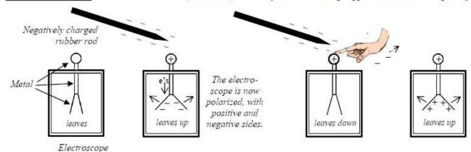
When a negatively charged object comes close, free electrons move away, down the metal of the electroscope to the thin metal leaves. Since both are negative, the leaves and repel each other, flying apart.
