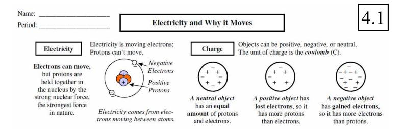
Any two charges feel a force between them. Electric force depends on the types of charges, the distance between the charges, and the amounts of the two charges.
